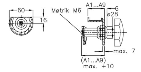
Door + frame thickness = 17-25 Measure type = A1
